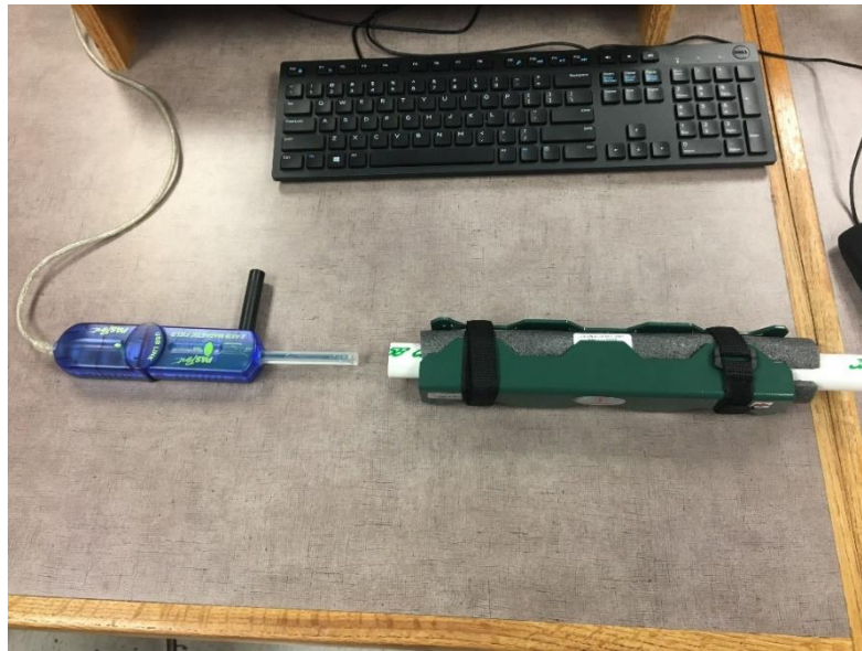
Image 1: 2 axis Magnetic field sensor used to measure gauss power of magnets
