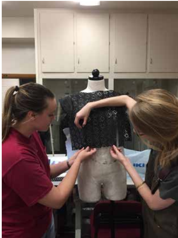
Fig. 3. The authors assemble 3-D printed top with welding glue.
