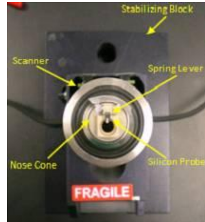
Figure 5: AFM large scanner assembly.
