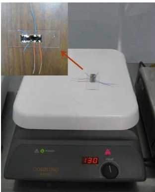
Figure 6: Heat plate for wire bonding.
