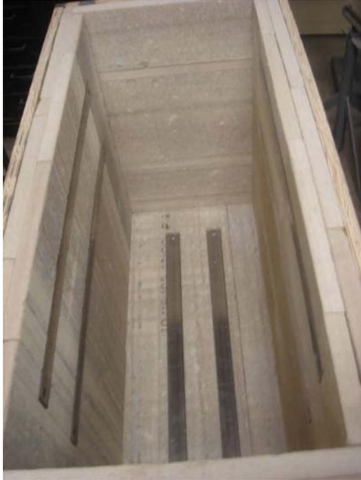
Figure 3. Strip Heaters for Start-Up
