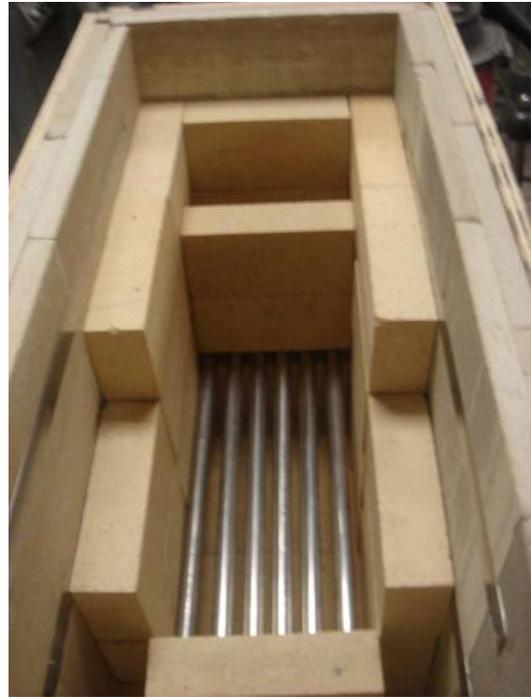
Figure 4. A Tube Bank within Gasifier
