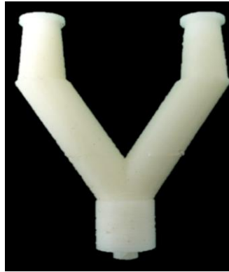
Figure 8. This figure is a photo of prototype eight. The uPrint SE Plus printer created a prototype made of ABS. The material was too rough and caused overflowing of the hydrogel mixture.
