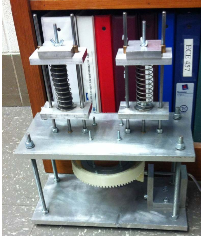
Fig. 20: Mass Spring System Teaching Aid [3]
