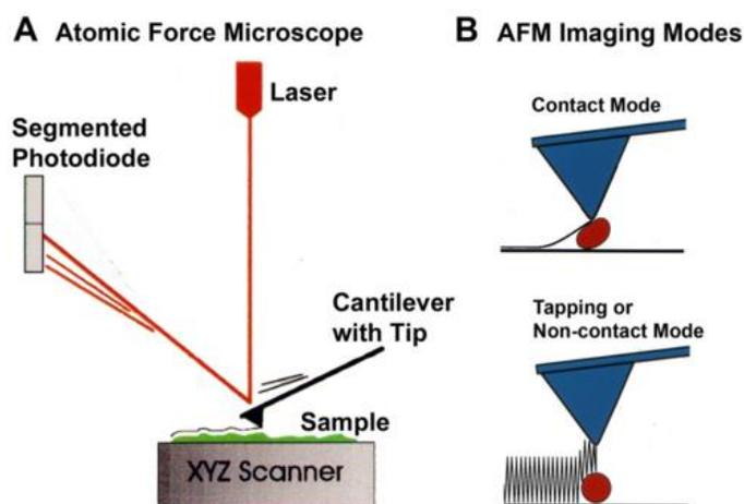
Figure 1. AFM Mechanics [4]
