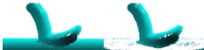
Figure 1. Using RANSAC, background surface was detected and removed.
