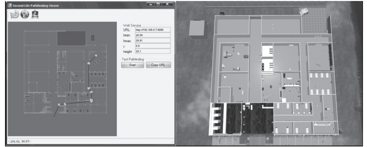
Figure 5. A visual tool for inspecting the bounding boxes with which our web service is generating a path and the corresponding SL hospital on the University of Arkansas island (right).
