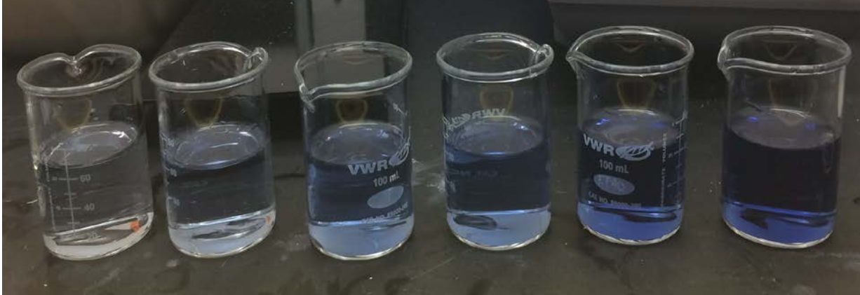
Figure 3. Samples of 0.1, 0.2, 0.4, 0.6, 0.8, and 1.0 mg per L of P reduced with ascorbic acid
