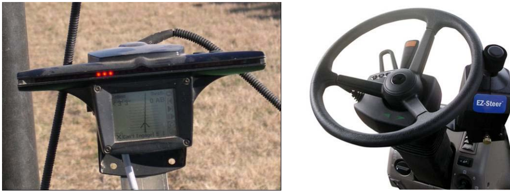
Fig. 1. Light-bar (left) and assisted-steering (right) guidance systems.
