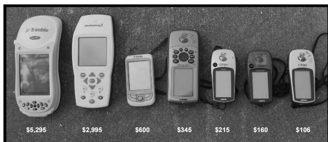
Figure 1. The seven GPS receivers tested in this study were Trimble GeoXH, Trimble GeoExplorer3, Trimble Juno, Garmin GPSMAP 76CS, Garmin eTrex Vista, Garmin eTrex Legend, Garmin eTrex (left to right with their cost shown below).
