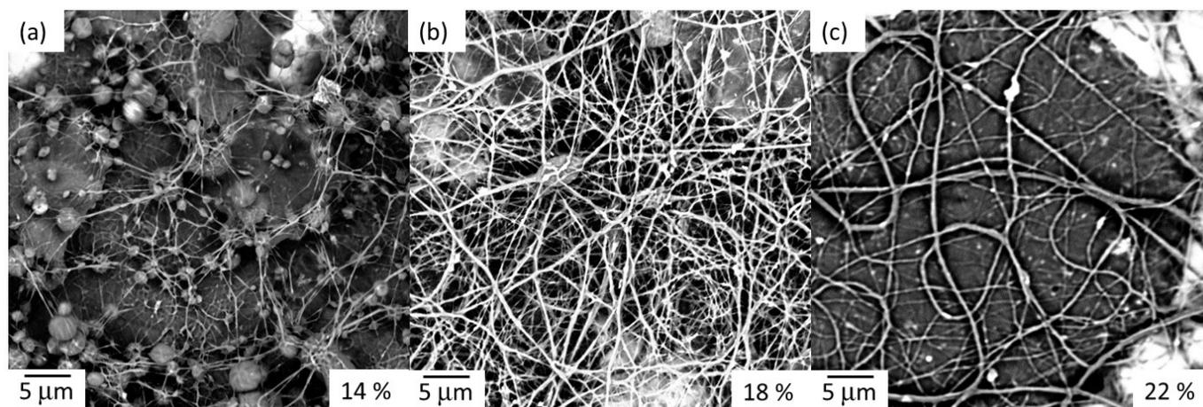
Figure 2. SEM images ( $45\mu\text{m} \times 45\mu\text{m}$ ) of electrospun fibers produced from three different PEO solution concentrations (a) 14%, (b) 18%, and (c) 22%. For each concentration, the fibers were produced using an 18 kV tip potential, 15 cm tip-collector separation, and a 0.65 mL/hr solution pumping speed.
