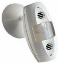
non-audible, high frequency (40kHz) to sense Doppler shifts caused by motion in the space. The ultrasonic is more sensitive to small motion and does not rely on line of sight for detection. If both sensors have not detected any motion for the set timeout period, the lights will be turned off.
