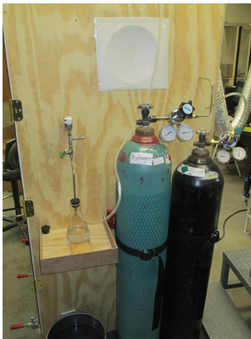
**Figure 3.** Shown are the strapped cylinders, product vessel, and weak explosion vent.
