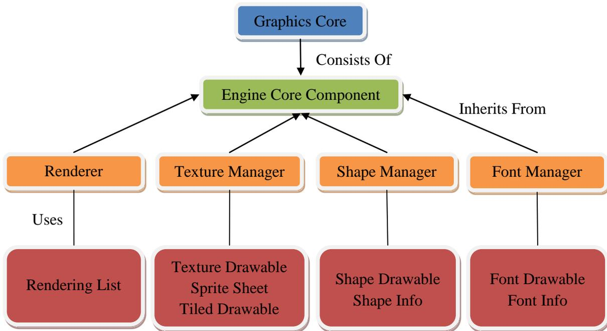
**Figure 3: Breakdown of the Graphics Core**
