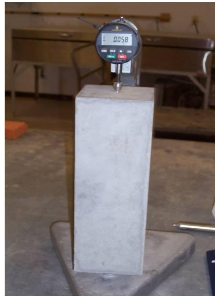
Figure 2 Shrinkage Testing Prism
