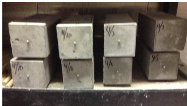
Figure 3 Shrinkage Specimens Storage
