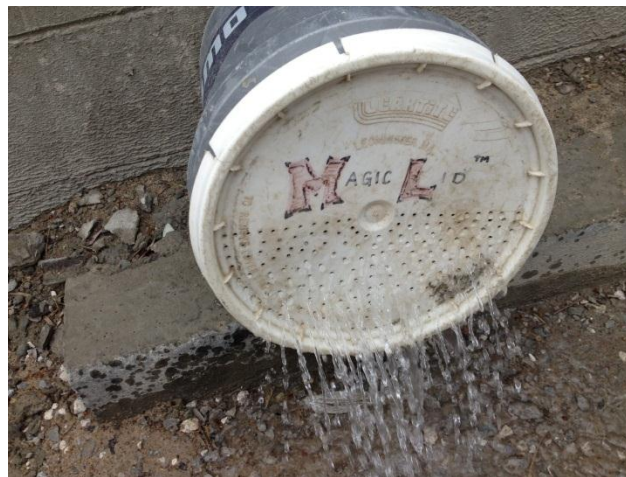
Figure 1 Removal of Excess Water From FLWA
