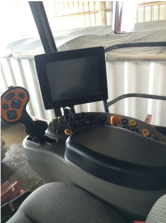
Figure 2. AFS Pro 600 Display (left) and AFS 262 Receiver (right).
