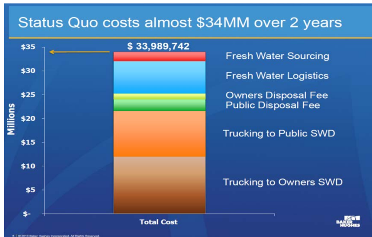
Figure 13. Analysis of typical costs for water acquisition and treatment in the fracing industry 12
