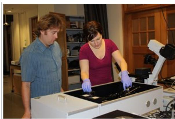
Colin Heyes, left, and research collaborator Nela Durisic align the optical components of a microscope to improve its sensitivity to detect single quantum dots.
