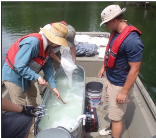
Figure 9. Method for distributing chemical fertilizer in lakes. The number of bags of each fertilizer is determined from the fertilizer calculator and the fertilizer is dissolved shipboard and pumped slowly into lake as the boat travels around the entire lake.
