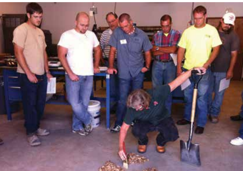
CTTP instructor Mary Fleck demonstrates one method of dividing an aggregate sample for testing.
