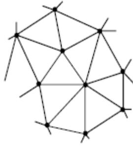
Figure 5.3: Unstructured mesh discretization
