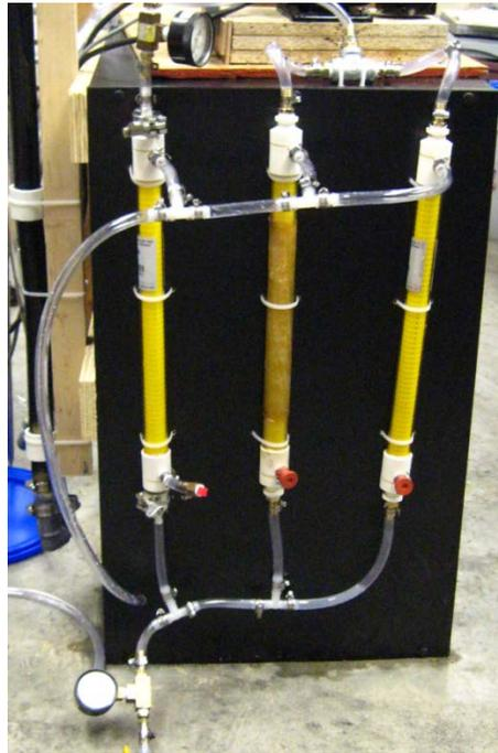
**Figure 1.** Parallel ultrafiltration membranes.
