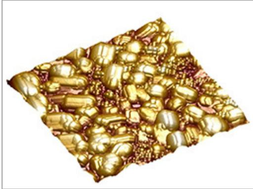
This image shows silica nanoparticles on the surface of polytetrafluoroethylene, a widely used polymer.
