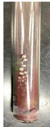
**Figure 5.** Sn pellets and P powder in vacuum sealed quartz tube.
