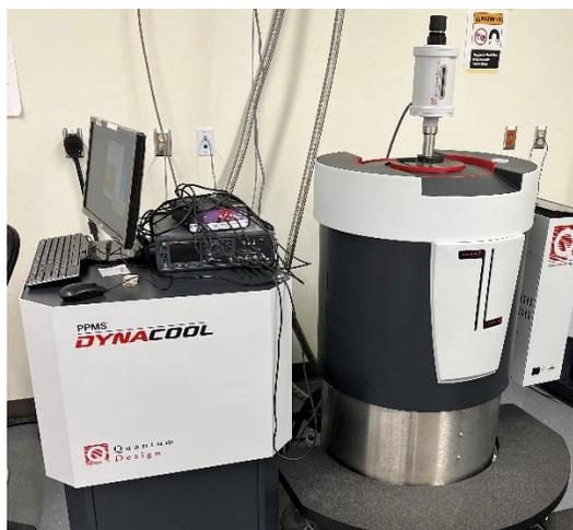
**Figure 11.** Physical Properties Measurement System (PPMS) by Quantum Design. This is the mechanism used to obtain the measurements for the physical properties of the crystal.
