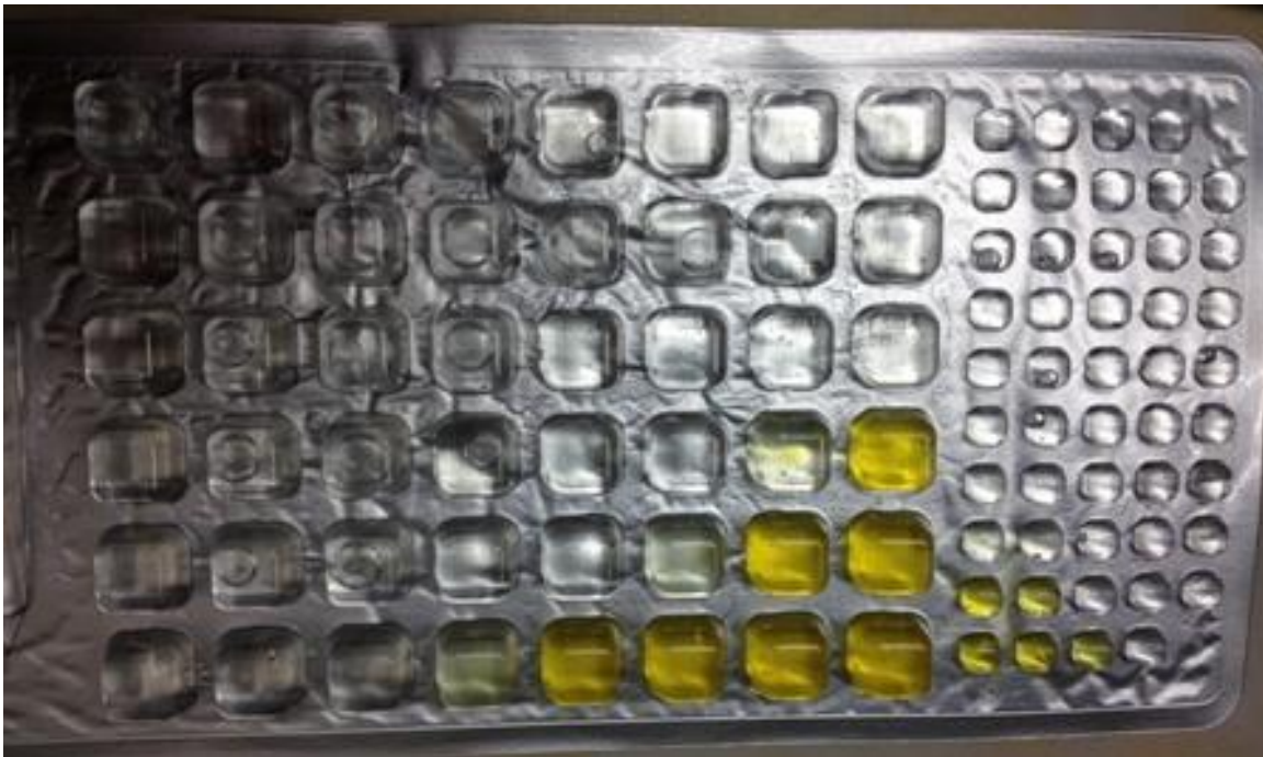
Figure 2.1: Tray incubated at 30°C (86°F) after 21 hours of incubation. At this time, 10 large wells and five small wells indicate a positive hit.
