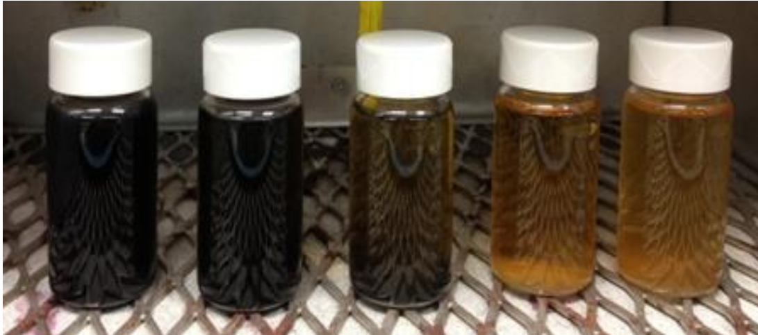
Figure 1.2: Sample after 24 hours of incubation at 22°C (71.6°F). The vial on the far right exhibits essentially no color change. The color change which indicates positive results is quite obvious by comparison.
