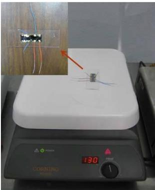
Figure 6: Heat plate for wire bonding.
