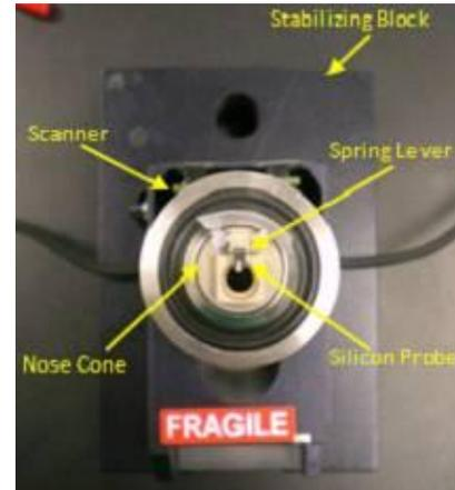
Figure 5: AFM large scanner assembly.
