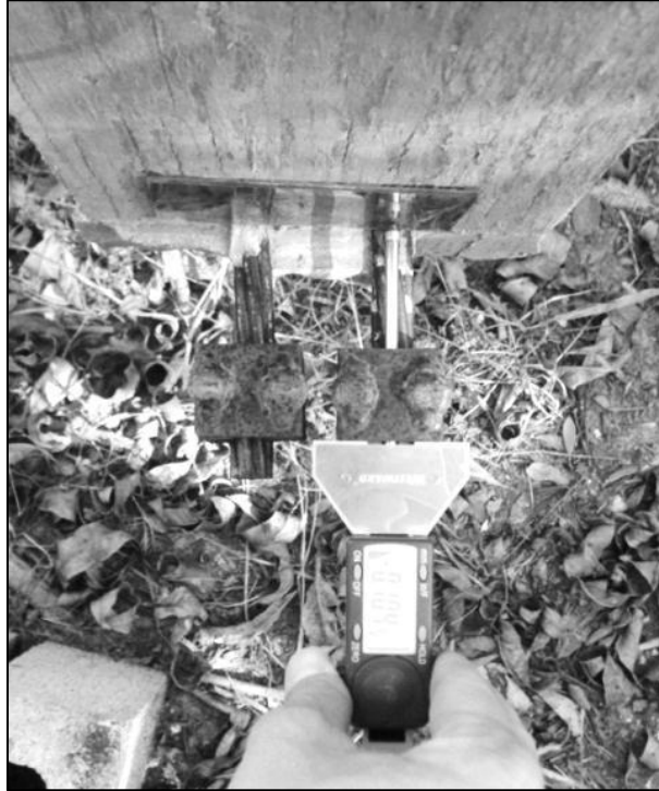
Figure 1: End Slip Measurement
