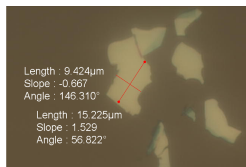
Figure 2: A satisfactory section of BP is measured to be approximately 9μm by 15μm. It appears uniform, and its color suggests ideal thickness.
