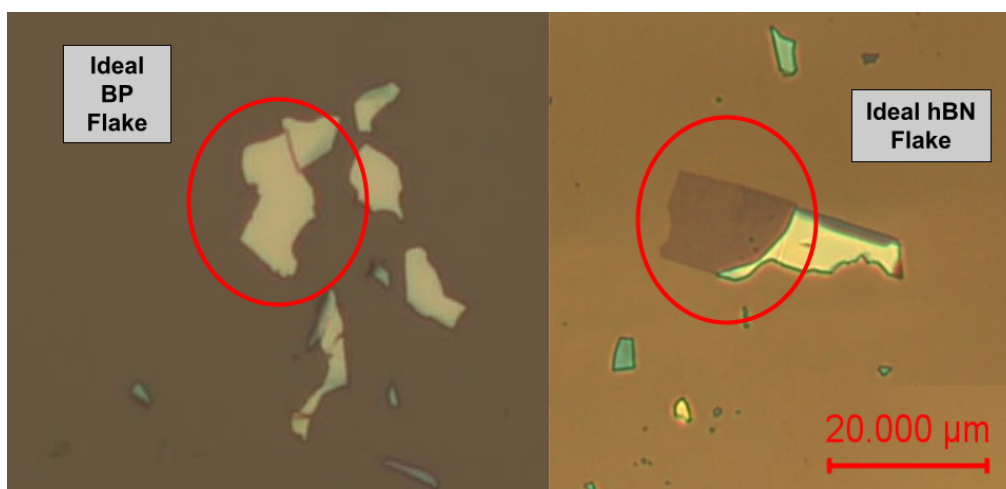
Figure 1: Two candidate flakes, BP (left) and hBN (right) are identified by their color, size, and uniformity.
