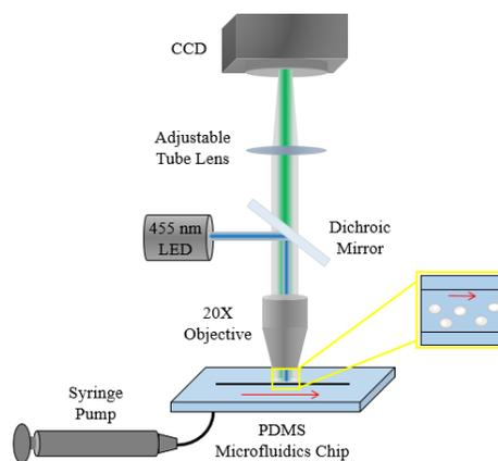
Figure 2. Schematic image of epi-illuminating fluorescence microscope.
