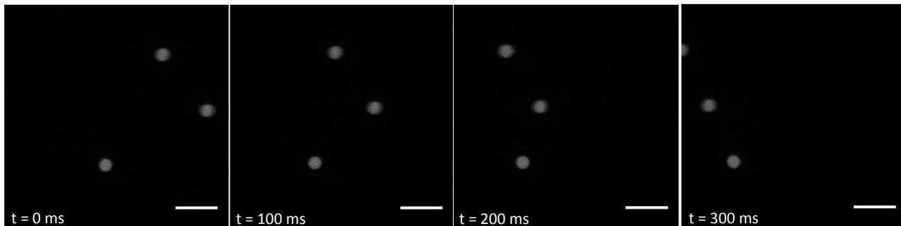
Figure 5. Consecutive images of bead flow across the focal plane of a 4X objective in a 500  $\mu\text{m}$  channel. Images were captured at 5 ms exposure time and 0 dB gain. Scale bar is 50  $\mu\text{m}$ .
