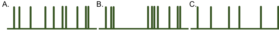
Figure 2.1: Types of photon sources. A. Coherent B. Bunched C. Antibunched source. The vertical bars represent photon detection events against time (horizontal axis). For coherent photon sources (A), the vertical bars i.e., the photon detection events occur at random time intervals whereas for bunched photon sources (B), the photons arrive in a bunched fashion. Similarly, for antibunched photon sources (C), like single photons, detection probability of two or more photons arriving at the same time is very small (close to zero for good single photon sources).
