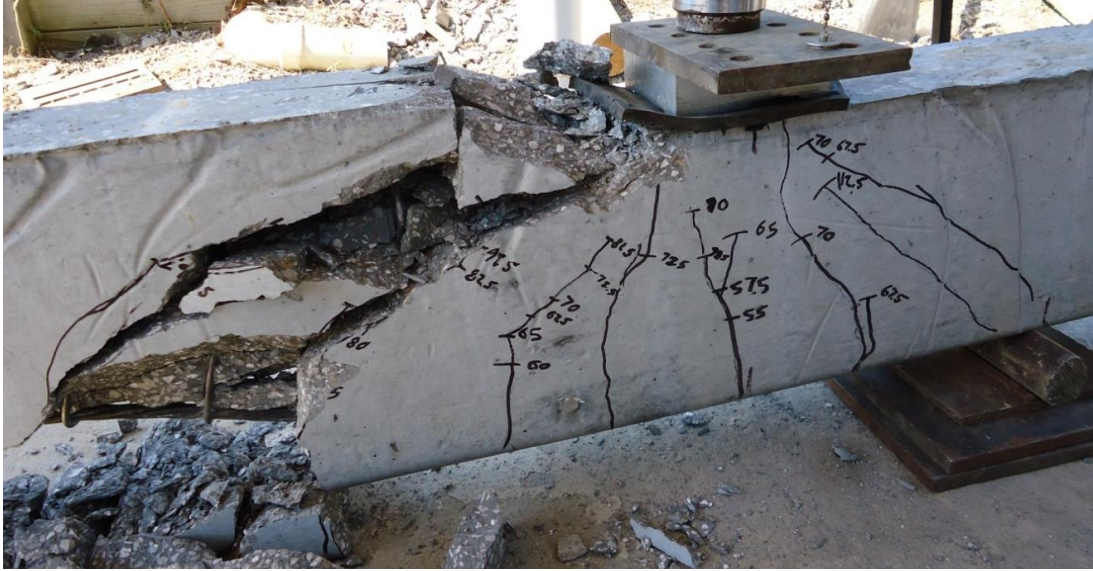
Figure 4. Limestone 1 Live End Test – Typical Flexure-Shear Failure
