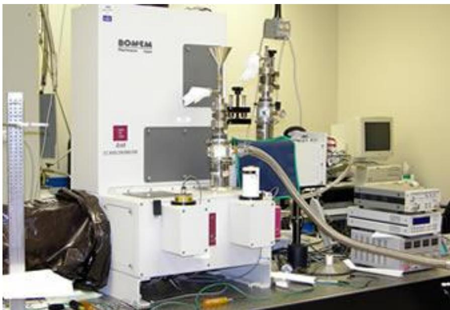
**Figure 3.3** The Bomem DA8 FTIR spectrophotometer
