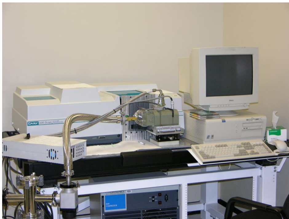
Figure 3.1 The Varian Cary 500 spectrometer
