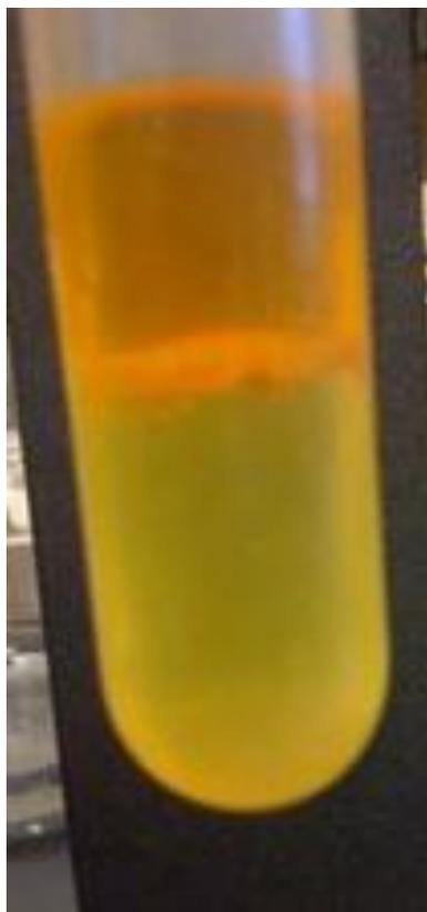
**Figure 6:** Liquid-Liquid Separation of Lycopene from Bitter Melon Aril Using Extraction Method 2.
