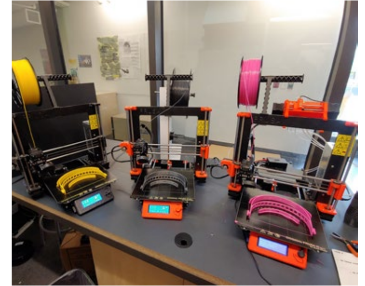
Prusa 3D printers making the pieces for face shield frames.
