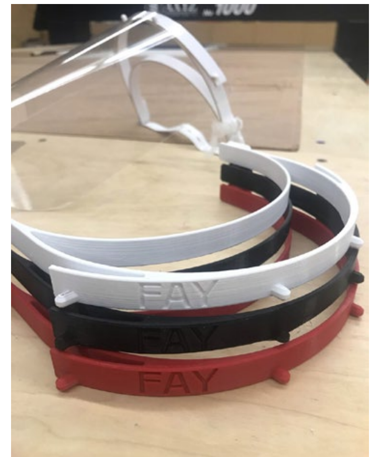
The Fay Jones School staff 3D printed face shield frames for the school community in red, white and black. Some assembled face shields are shown above, and the 3D printed frames are shown in the bottom right photo. Photos courtesy of Randal Dickinson.
