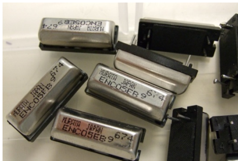
Figure A3: Rate Gyros Designed for Use in a MEMS Device [11].
