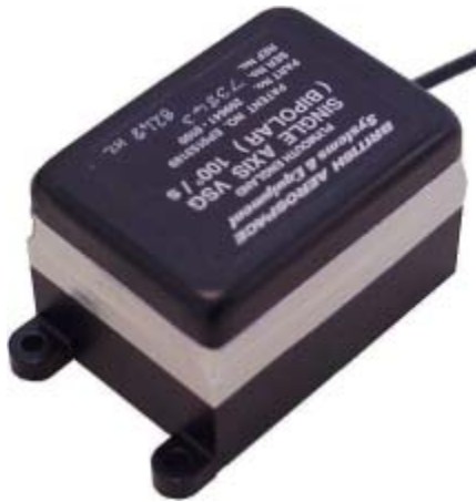
Figure A4: Rate Gyro Similar to One in Control Circuit [18].
