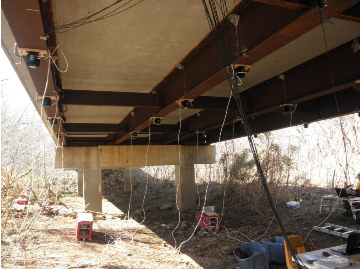
Figure 3. Equipment set up under the bridge span being analyzed.
