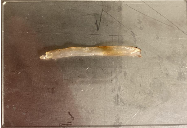
Figure 1: Non-uniform dispersion based Nafion sample.
