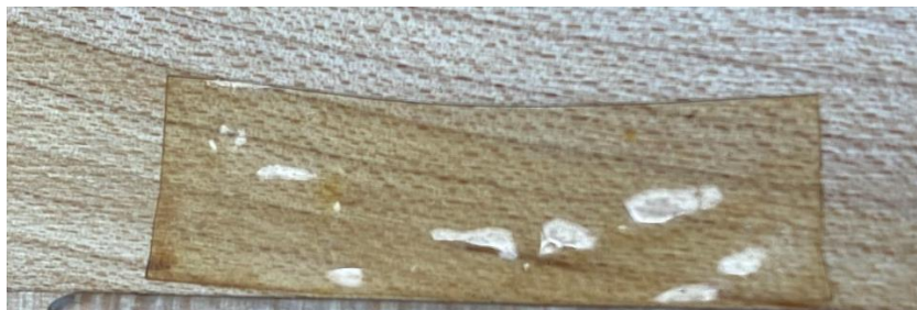
Figure 2: Sheet based, hand cut Nafion sample.
