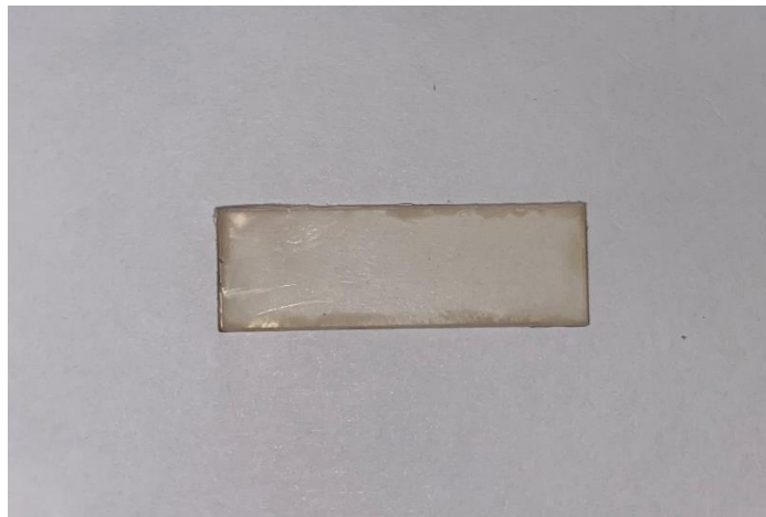
Figure 4: Sheet based, CO 2 laser cut Nafion sample.
