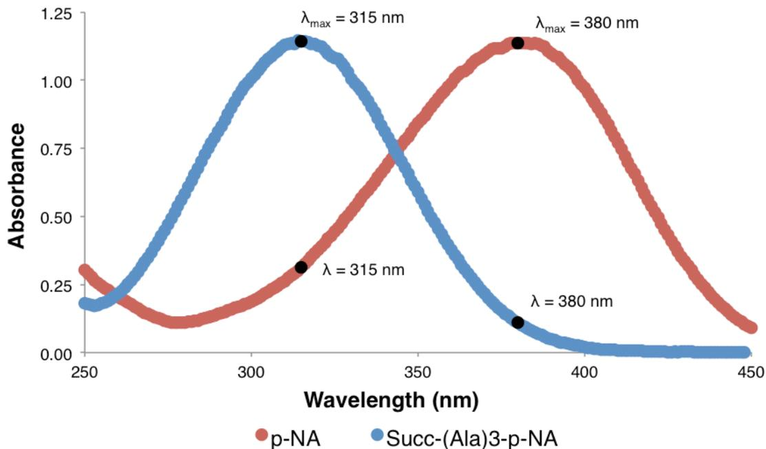
**Figure 4:** Absorbance spectra measured for 1000  $\mu\text{M}$  Succ-(Ala)<sub>3</sub>-p-NA and 1000  $\mu\text{M}$  p-NA. The maxima are labeled as well as the corresponding measurement on the non-dominant spectra showing the overlap of the absorbance measurements due to the combination of unreacted Succ-(Ala)<sub>3</sub>-p-NA substrate and p-NA product that would be present in microdialysis dialysate.
