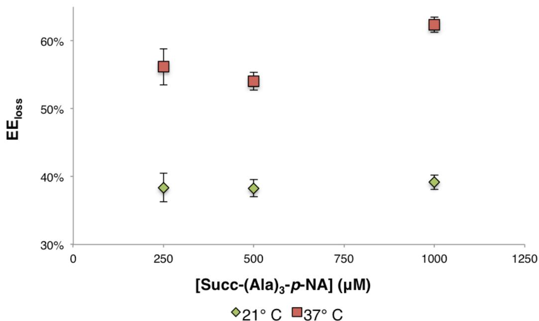
**Figure 10:** Succ-(Ala)<sub>3</sub>-p-NA concentration vs. EE<sub>loss</sub> of microdialysis delivery of various concentrations of Succ-(Ala)<sub>3</sub>-p-NA into triplicate 2 mL elastase solutions (pH=7.4) at 1.0 unit/mL. Solutions allowed to equilibrate for 15 mins prior to a 7 min collection at 1.5 μL/min flow rate. Data represented as mean ± SD (n=3).
