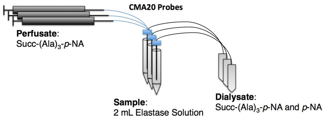
**Figure 3:** Microdialysis setup used in these experiments. Three syringes, loaded with Succ-(Ala)<sub>3</sub>-*p*-NA solutions, connect to three separate probes submerged in elastase solutions. The outlets empty into separate microcentrifuge vials.
