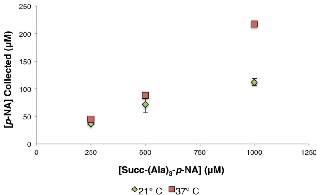
**Figure 11:** Succ-(Ala)<sub>3</sub>-p-NA concentration vs. product (p-NA) collected in dialysate following delivery of various concentrations of Succ-(Ala)<sub>3</sub>-p-NA into triplicate 2 mL elastase solutions (pH=7.4) at 1.0 unit/mL. Solutions allowed to equilibrate for 15 minutes prior to a 7 min collection at 1.5 μL/min flow rate. Data represented as mean ± SD (n=3).
