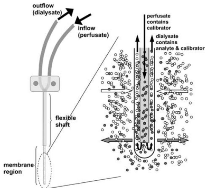
**Figure 1:** Diagram depicting diffusion-based movement of analyte using a microdialysis probe. Perfusate enters through the inlet and out of the inner tube where it can then interact with the semi-permeable membrane either diffusing into the solution or continuing into the dialysate. Analyte from the solution diffuses into the probe and is carried into the dialysate through the outlet tubing into a collection vial.<sup>3</sup>
