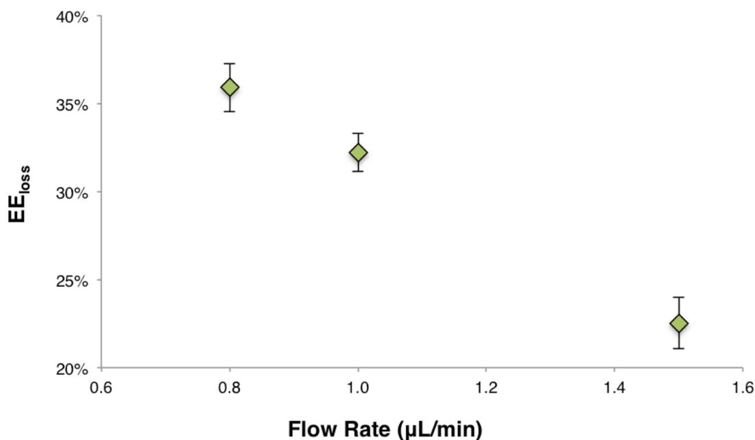
**Figure 7:** Flow rate vs  $EE_{\text{loss}}$  of a microdialysis-based delivery of 1000  $\mu\text{M}$  Succ-(Ala)<sub>3</sub>-*p*-NA eluted at 0.8, 1.0, and 1.5  $\mu\text{L}/\text{min}$  flow rates for 12.5, 10, and 7 min respectively into a 2 mL solution of 10 mM PBS (pH=7.4) at 21° C . There was no Elastase enzyme present in the samples. Data represented as mean  $\pm$  SD.
