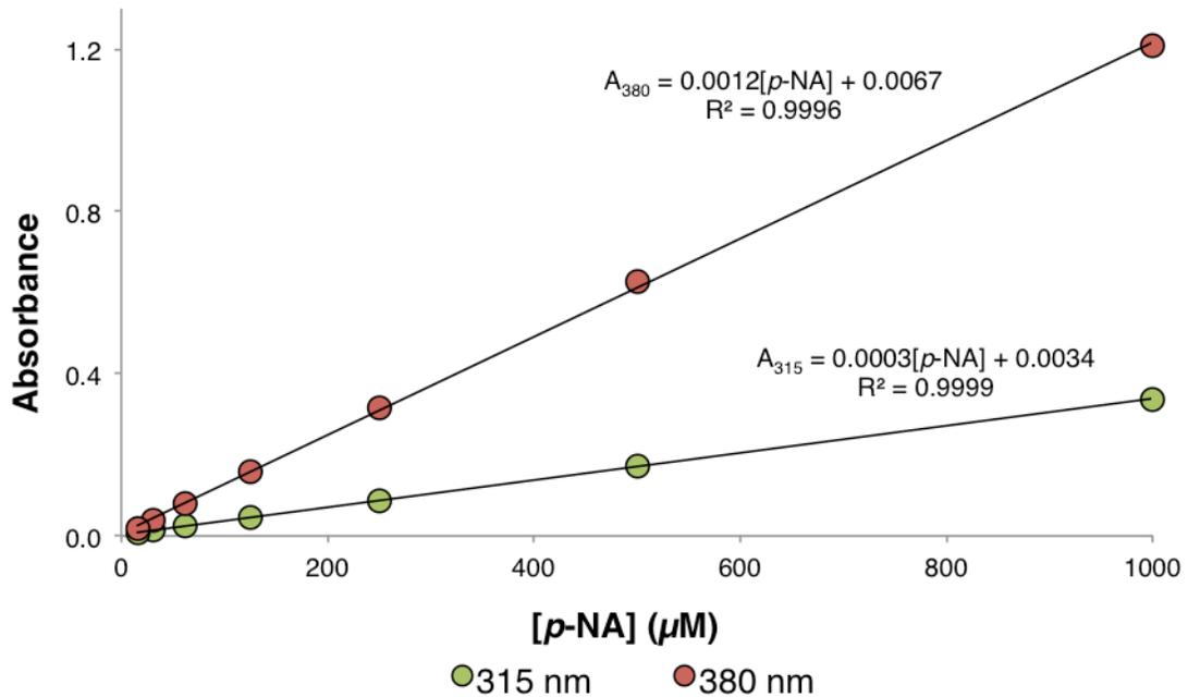
**Figure 6:** Calibration curve formed from 1000, 500, 250, 125, 62.5, 31.25, and 15.625 μM standards of p-NA in 10 mM PBS (pH=7.4). Data points represented as mean absorbance measurements at 315 and 380 nm using a NanoDrop 2000c (n=3).
