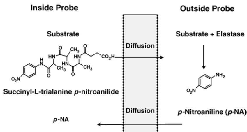
**Figure 2:** Diagram depicting a microdialysis probe in "Delivery" mode. The substrate (Succ-(Ala)<sub>3</sub>-*p*-NA) is perfused through the probe so as to diffuse into a solution of elastase. The metabolic product (*p*-NA) is then diffused back into the probe as dialysate.<sup>4</sup>
