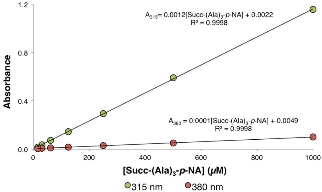
**Figure 5:** Calibration curve formed from 1000, 500, 250, 125, 62.5, 31.25, and 15.625 μM standards of Succ-(Ala)<sub>3</sub>-p-NA in 10 mM PBS (pH=7.4). Data points represented as averaged absorbance measurements at 315 and 380 nm using a NanoDrop 2000c (n=3).
