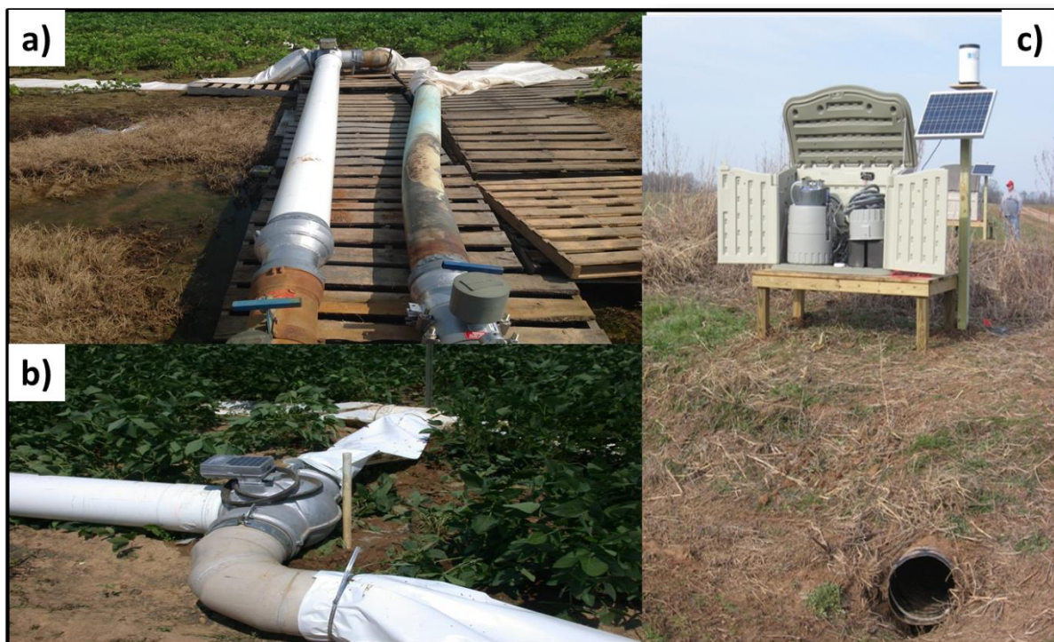
Fig. 2. Irrigation flow meters (a), surge (b) and automated runoff monitoring station utilized to measure irrigation flow, automatic distribution of flow and tail water loss from irrigation.
