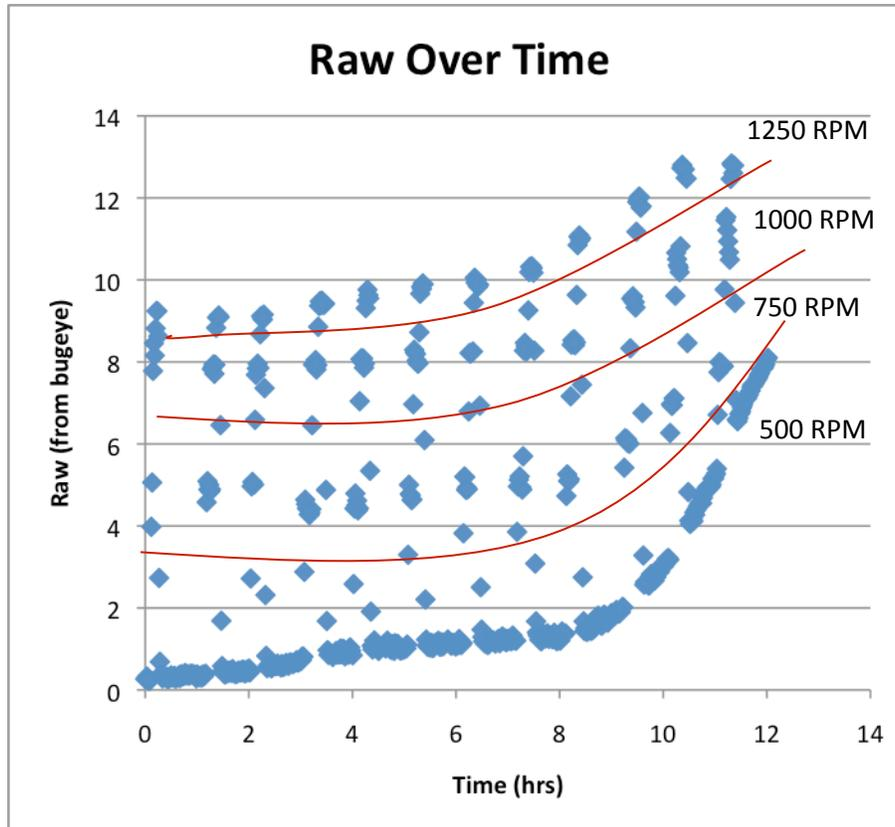
Figure 3: Plot of the raw OD data from the BE2100 “BugEye” OD probe over time during the fed-batch fermentation of *E. coli*; the baseline growth curve represents the bioreactor stirrer at 500 RPM, while the points above the baseline represent an increase in the RPM of the stirrer.
