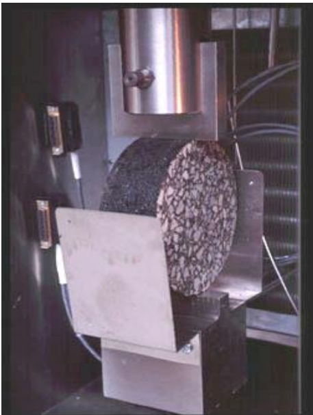
Figure 6 – Indirect Tensile Strength Test (AASHTO T322, from https://engineering.purdue.edu/ )
