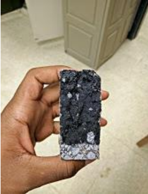
Figure 5 – SC(B) tested sample.
