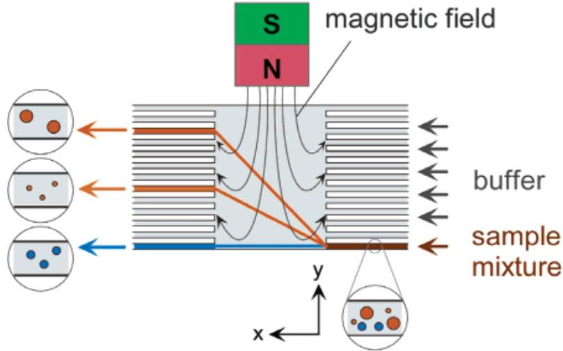
**Figure 4.** Diagram of the magnetophoretic separation chamber for the free-flow magnetophoretic chip<sup>10</sup>
