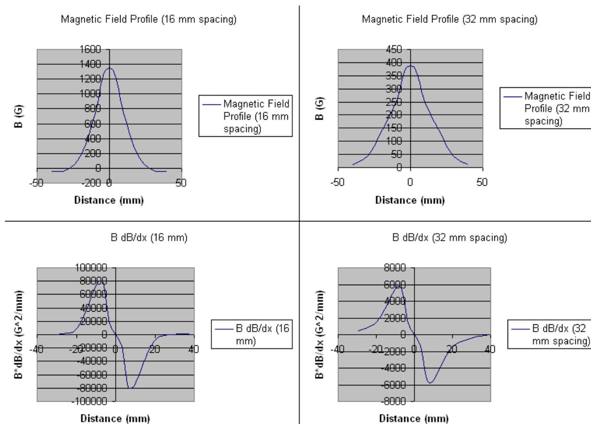
**Figure 13.** Magnetic measurements at 16 and 32 mm spacing
