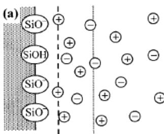
**Figure 1.** Diagram of ion interaction in EDL
