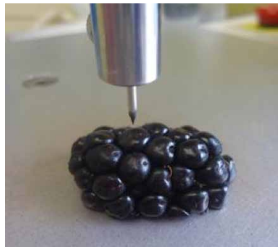
Fig. 2. Skin drupelet penetration measurement procedure utilizing a probe of 1 mm in diameter.
