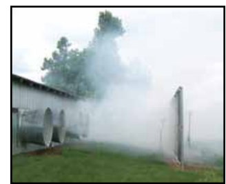
Figure 8. Smoke test on wind pattern generated by the tunnel fans
