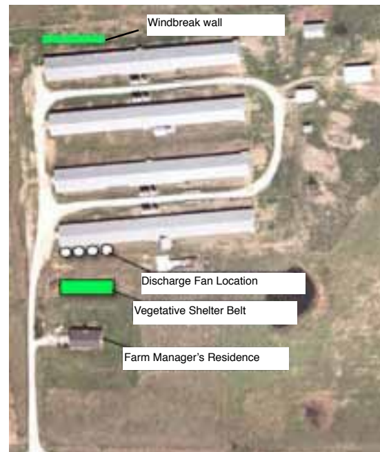
Figure 1. Aerial photos of the Applied Broiler Research Farm where this project is implemented. This photo shows the location of discharge fans, vegetative shelter belt installed and the structural windbreak wall installed.
