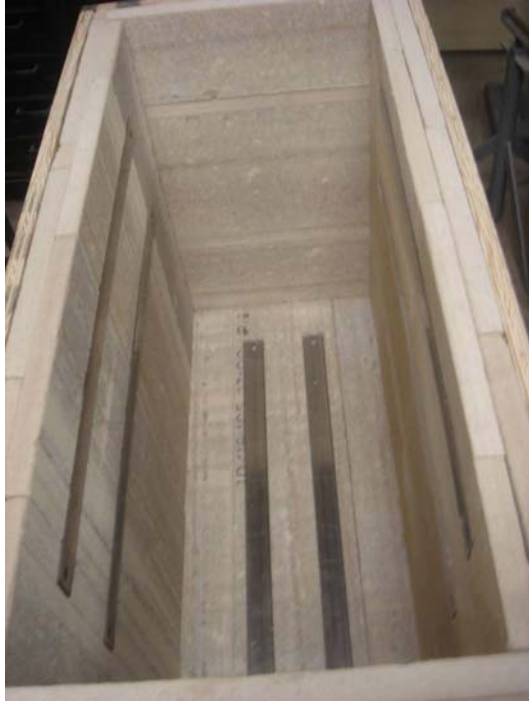
Figure 3. Strip Heaters for Start-Up
