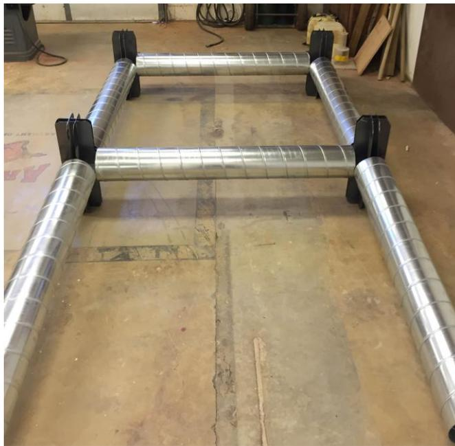
*Figure 11. Two-story plane frame prototype structure with 5' members.*
