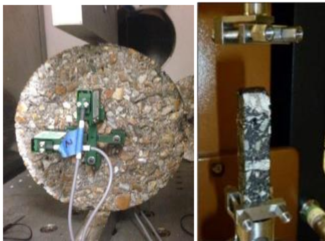
Figure 1: Dynamic modulus configurations: indirect tension (center), torsion bar (right) (Yang et al. , 2015).
