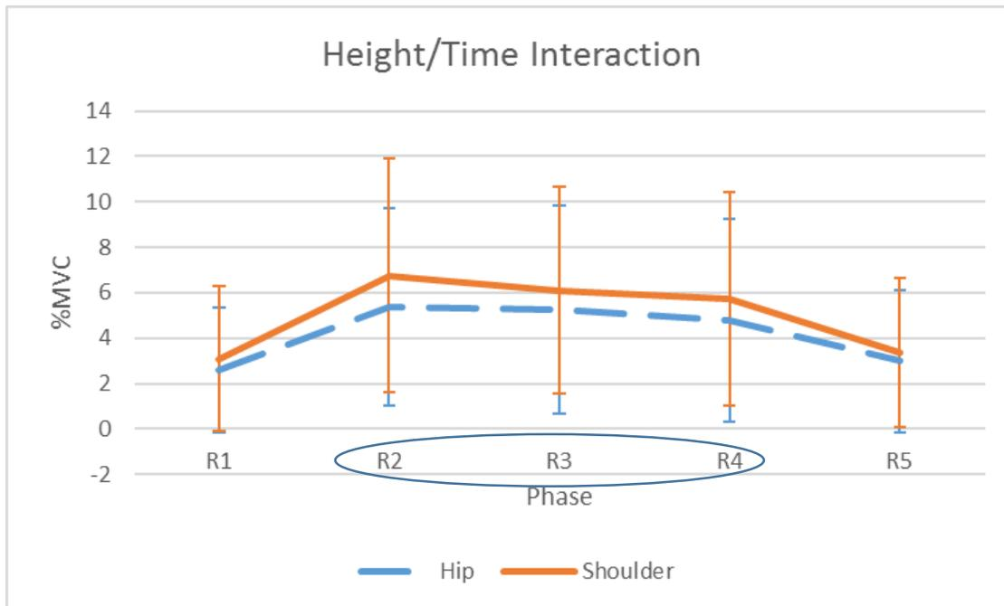
**Figure 2. Percent maximum voluntary contraction (%MVC) of peak EMG values for shoulder and hip level reaches. The circled phases demonstrate where there was a significant difference between muscle activity during the hip and shoulder reach heights.**
